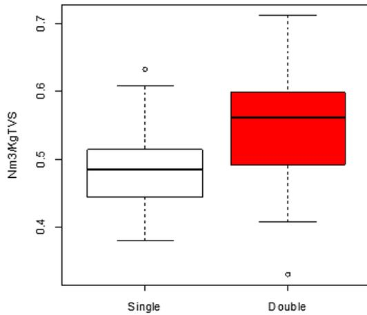
**Fig. 2** SMP obtained in single and two stage anaerobic digestion
