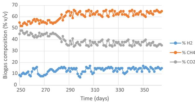
**Fig. 3** Biogas composition of the two stage AD (days 250–365)
