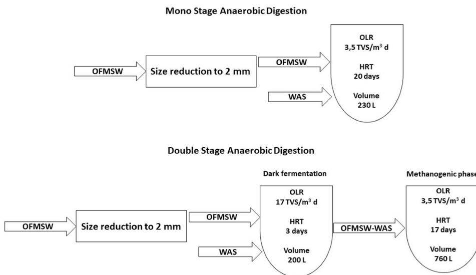
and OLR, together with pH, are very important parameters for the hydrogen and methane productions in continuous mode. Very low HRT comports the wash out of the reactor, which means that all the active microorganisms escape out from the reactor. On contrary, through high OLR it is possible to cause a decrease of pH as consequence of the overloading of the reactor. These conditions favour an overproduction of organic acids and of hydrogen [21, 22].
